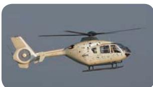
Eurocopter EC135 equipped with TURBOMECA ARRIUS
